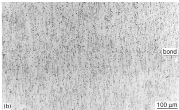
Figure 2 Joint microstructures produced on bonding (a) MA956 and (b) PM2000 at 1190 °C, 4 MPa, 30 min using the iron foil (2605 S2).
