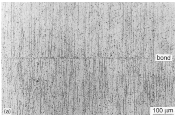
Figure 3 Joint microstructures produced using a 2 μm sputter coat at 1190 °C, 4 MPa, 10 min with (a) MA957 and (b) MA956.
