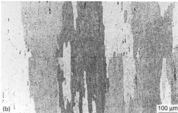
Figure 11 Micrographs showing the effect of isothermal heat treatment (at 1350 °C for 30 min) on TLP bonds made using MA956 with (a) foil interlayer and (b) sputter coat.
